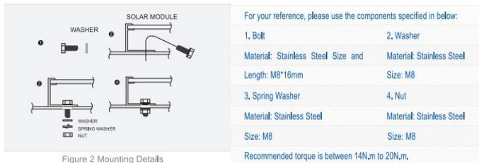
Figure 2 Mounting Details
